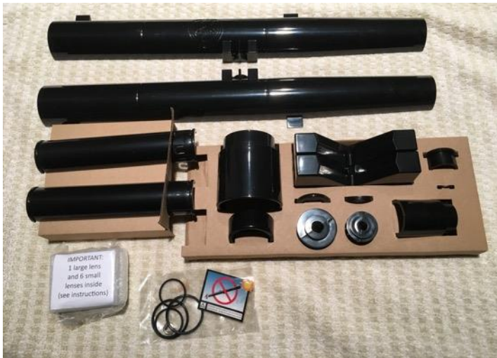
Figure 1. The Galileoscope can be disassembled into components. Shown are the lenses and the components that make up the focuser and body of the telescope.
