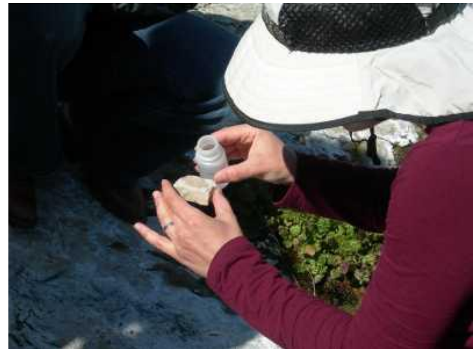
Dr. Dawn Cardace conducts an acid test on travertine deposit associated with serpentine at McLaughlin Natural Reserve, 2009. The acid fizzed readily, identifying carbonate minerals in the travertine deposit. Photo by Kathleen Scavone.
