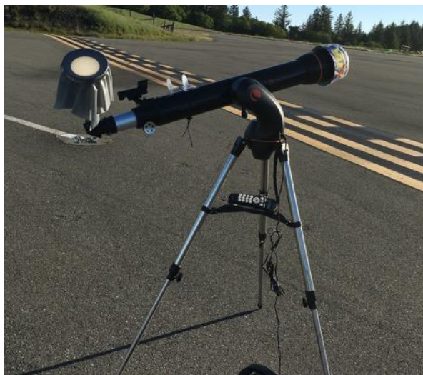
Figure 8. Sun funnel inserted into the diagonal of a 4-inch GoTo refractor telescope. (Image credit: GDW)
